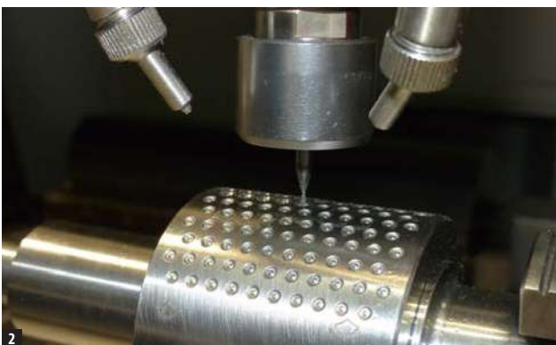
After switching to OSG's WXS-LN-EBD rib processing ball nose end mill, PräWEBA is able to increase tool life by an estimate of 125 percent in their production of metal stamping rollers.
