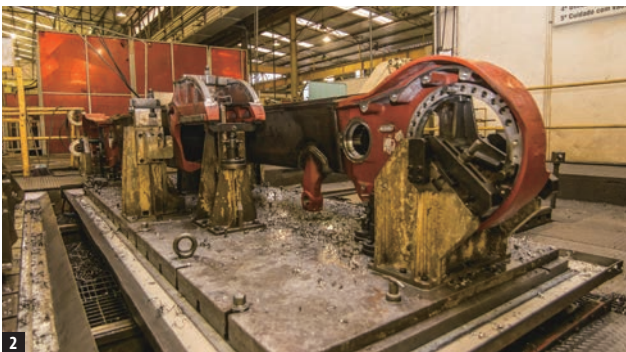
2 A track frame, which is a side-frame component of the bulldozer, waits for completion at Komatsu do Brasil's production plant in Suzano, São Paulo.
