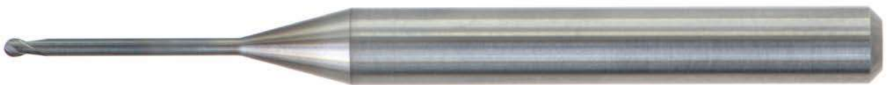
The WXS-LN-EBD is a 2-flute, long-neck ball nose carbide end mill designed for high-feed milling of hardened steels up to 65 HRC and stainless steels.
