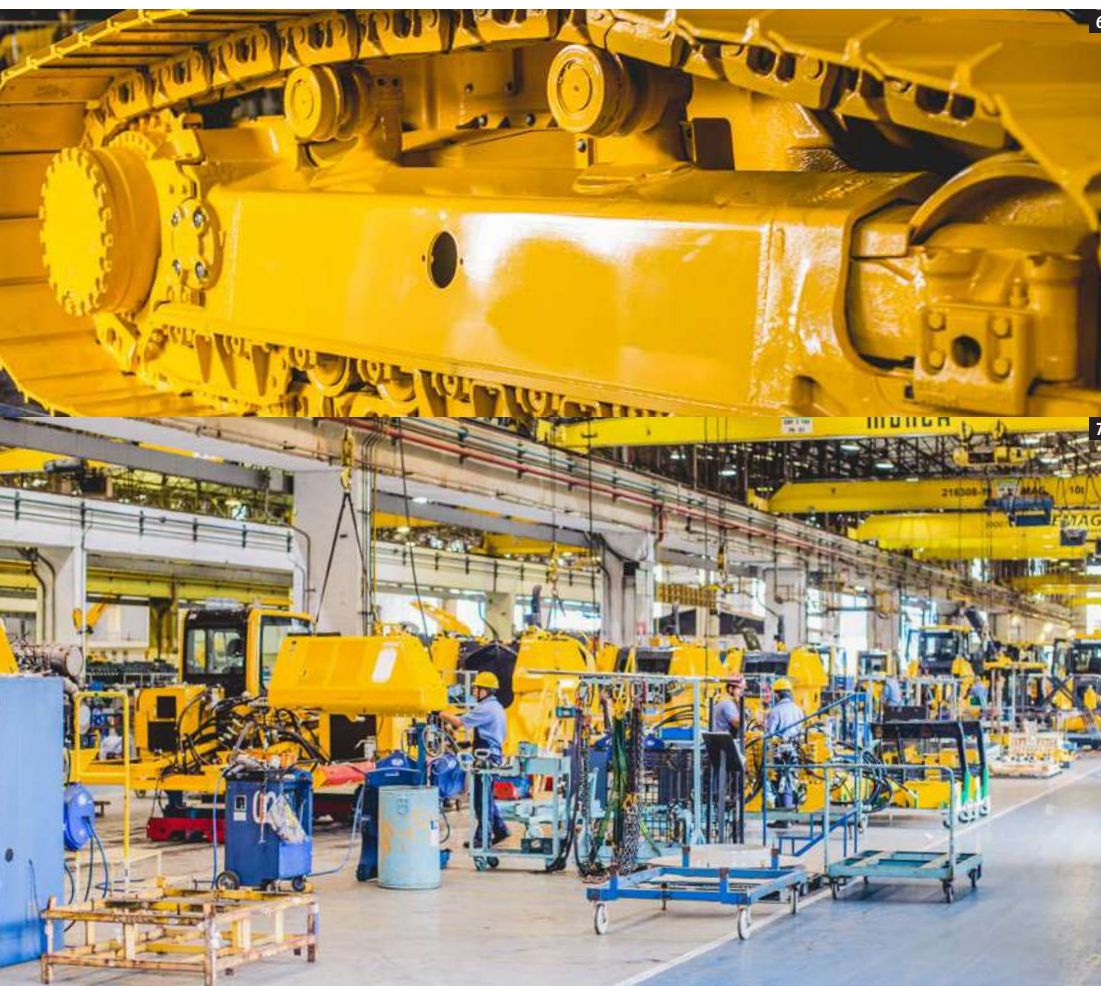
6. A close-up of a completed track frame on a bulldozer. The manufacturing of bulldozers requires a combination of processes, such as CNC machining, welding and powder coat painting involving skilled technicians as well as robotic support with automated assembly line.
