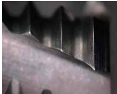
No.1 (after cutting 8,800 threads)
